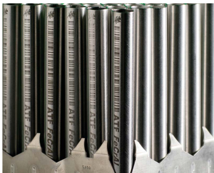
Figure 6: Mock-up of IronClad in a commercial fuel assembly.
