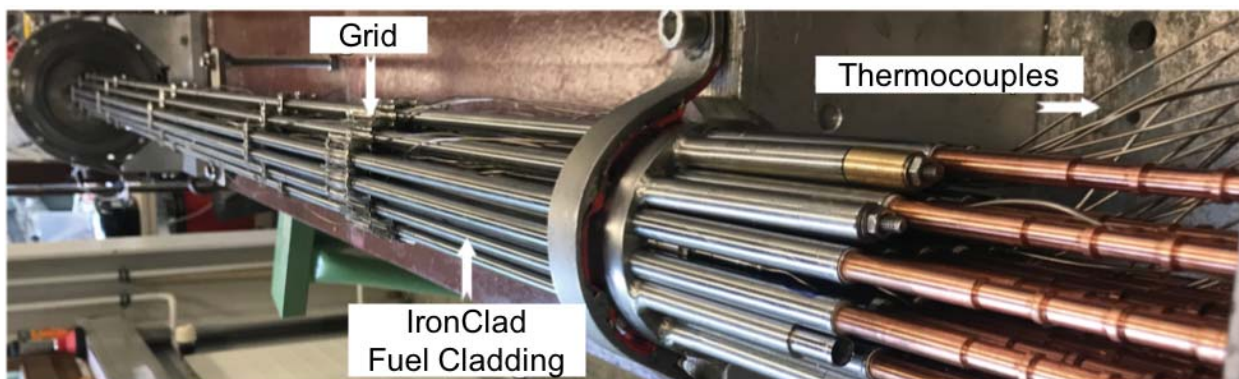
Figure 4: Assembly of QUENCH-19 test with IronClad rods at Karlsruhe Institute of Technology. The test assembly was heated using electrical heaters inside the cladding to simulate heat from radioactive decay while being subjected to high temperature flowing steam. The ~3h test reached a temperature of ~1400°C that is 500°C lower than what is experienced at much shorter time with oxidation-susceptible Zr-based cladding and produced at least an order of magnitude lower hydrogen gas.
