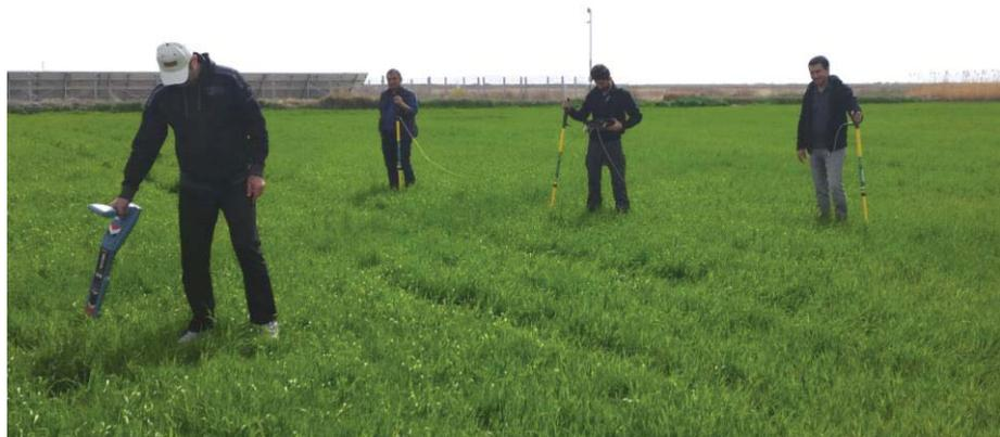
of the pipe to confirm which pipe has the defect. The Hexcorder Pro has 4 DCVG channels, allowing simultaneous gradient recording of any combination of the left, right, front and rear. The Hexcorder Pro can also record CIPS measurements at two different input impedances, 25
