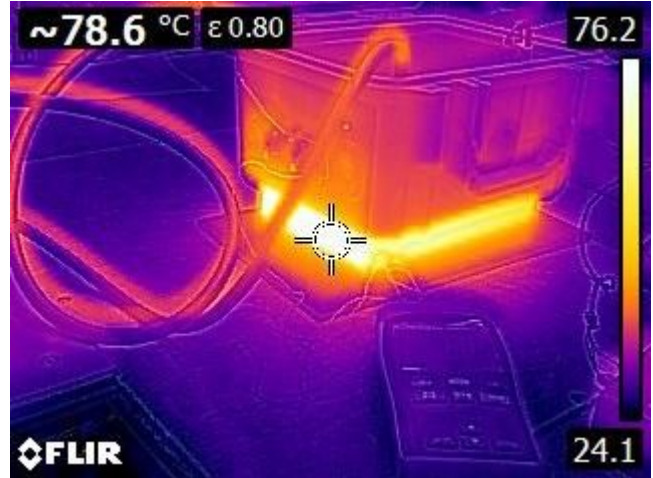
Figure 7 - Temperature at 200% of rated current
