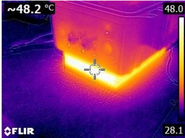
Figure 6 - Temperature at 110% of rated current
