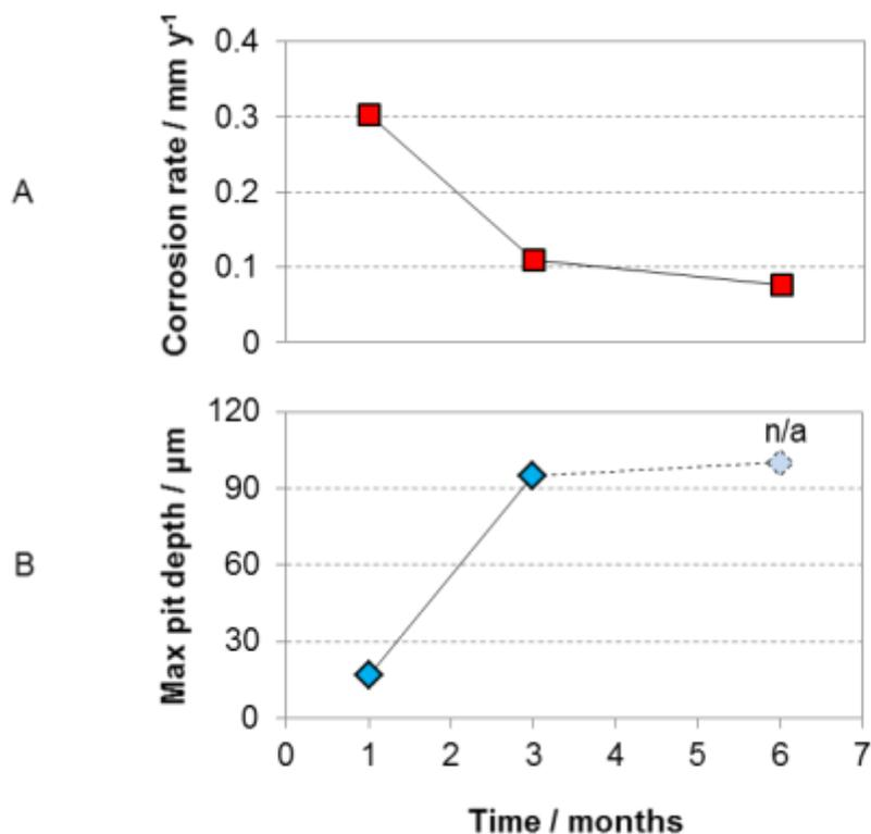
**Figure 9: A) Corrosion rate and B) maximum pit depth of UNS S31603 determined after exposure in the artificial LHD-23 geothermal brine at 175 °C**
