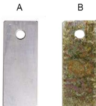
**Figure 10: UNS S31603 coupons appearance after 6 months of exposure in the artificial LHD-23 geothermal brine at: A) 100 °C and B) 175 °C**
