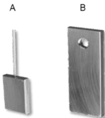
**Figure 1: Material sample preparation for: A) electrochemical and B) exposure tests**
