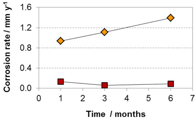
**Figure 5: Corrosion rates of UNS G41300 after exposure tests in the artificial LHD-23 geothermal brine at: (◆) 100 °C and (■) 175 °C**
