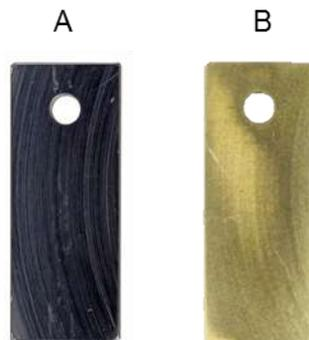
**Figure 15: UNS N08031 coupons appearance after 6 months of exposure in the artificial LHD-23 geothermal brine at: A) 100 °C and B) 175 °C**
