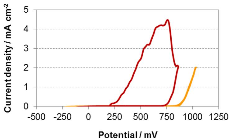
Figure 12: Temperature influence on typical anodic and cathodic polarization curves for high-alloyed stainless steel UNS N08031 in artificial LHD-23 geothermal brine at: (—) 100 °C and (—) 175 °C
