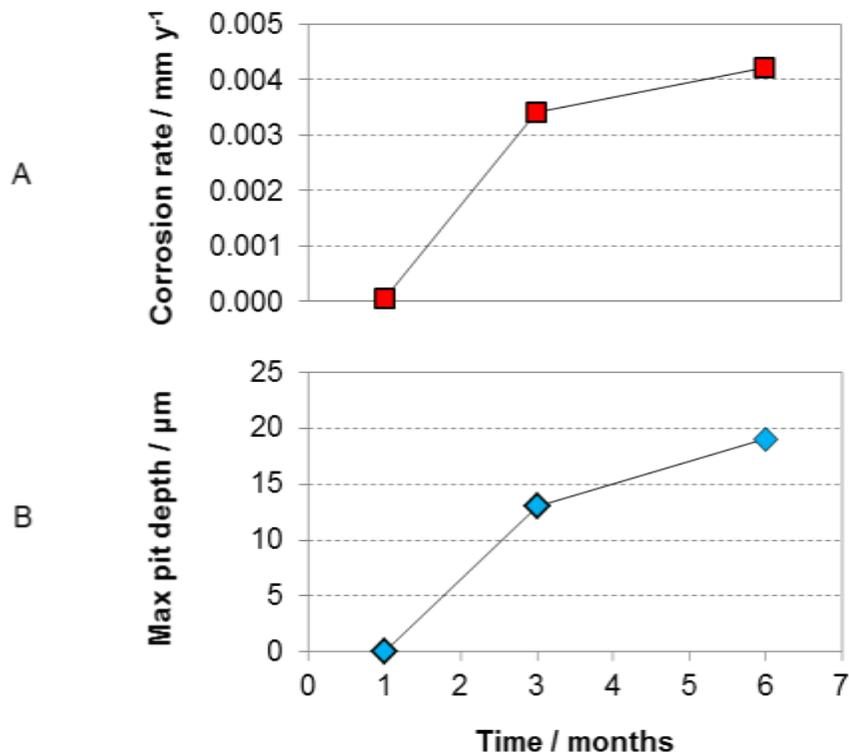
**Figure 14: A) Corrosion rate and B) maximum pit depth of UNS S31603 determined after exposure in the artificial LHD-23 geothermal brine at 175 °C**
