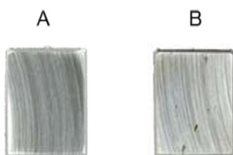
Figure 13: High-alloyed stainless steel UNS N08031 electrode appearance after cyclic polarization in the artificial LHD-23 geothermal brine at: A) 100 °C and B) 175 °C
