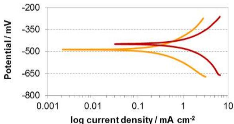
**Figure 3: Typical anodic and cathodic polarization curves for low-alloyed steel UNS G41300 in artificial LHD-23 geothermal brine at: (—) 100 °C and (—) 175 °C**
