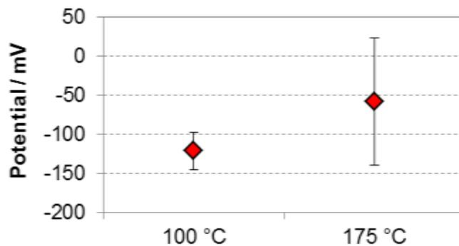
**Figure 6: Temperature influence on open circuit potentials of stainless steel UNS S31603 in the artificial geothermal LHD-23 geothermal brine**
