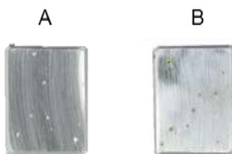
**Figure 8: Stainless steel UNS S31603 electrode appearance after cyclic polarization in the artificial LHD-23 geothermal brine at: A) 100 °C and B) 175 °C**
