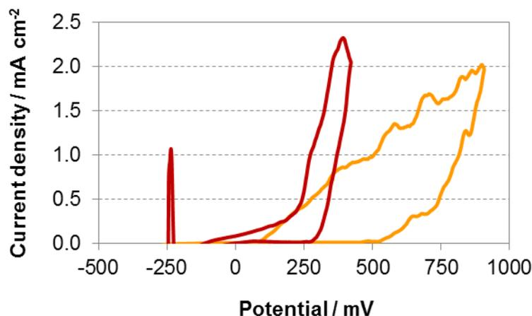
**Figure 7: Temperature influence on typical anodic and cathodic polarization curves for stainless steel UNS S31603 in artificial LHD-23 geothermal brine at: (—) 100 °C and (—) 175 °C**
