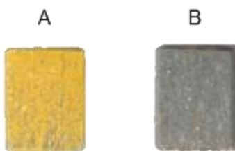
**Figure 4: Low-alloyed steel UNS G41300 electrode appearance after dynamic polarization in the artificial LHD-23 geothermal brine at: A) 100 °C and B) 175 °C**
