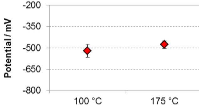
**Figure 2: Temperature influence on open circuit potentials of low-alloyed steel UNS G41300 in the artificial geothermal LHD-23 geothermal brine**
