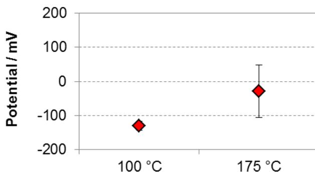
**Figure 11: Temperature influence on open circuit potentials of high-alloyed stainless steel UNS N08031 in the artificial geothermal LHD-23 geothermal brine**
